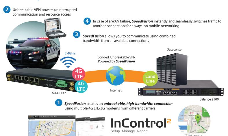
InControl 2 provides complete cloud-based device management, monitoring, and reporting and let you check vehicle speed, view cellular coverage, and
