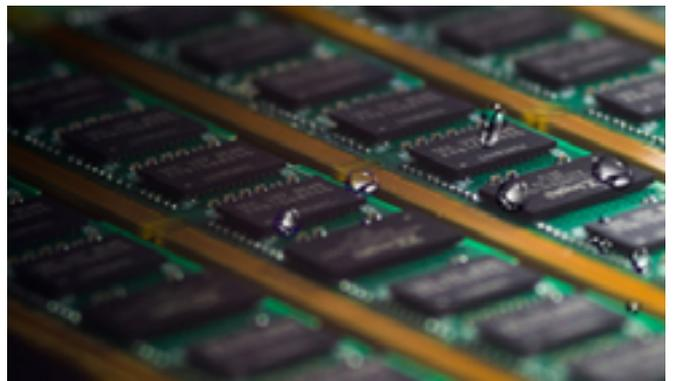
A protective layer of Parylene is applied to electronic circuits and modules, accessing spaces as narrow as 0.01 mm to shield against dust, chemical, extreme temperatures, moisture and corrosion. The coating film is formed by the chemical vapor deposition (CVD) process, and unlike dipping and spraying techniques, is completely pinhole free as the film conforms to any irregular shape, forming a vacuum-like environment to coat all components and points of failure.
