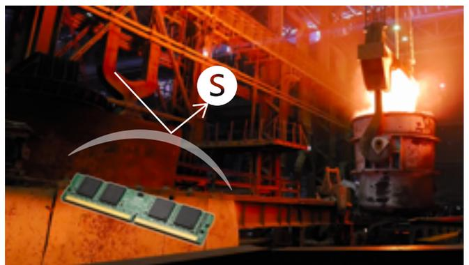
Ordinary silver resistors corrode and become non-conductive when exposed to sulfur. ATP DRAM modules use anti-sulfur resistors that repel the damaging effects of sulfur contamination, guaranteeing continued dependable performance for a long time and lowering the total cost of ownership by preventing unnecessary downtime and expensive component replacements.
