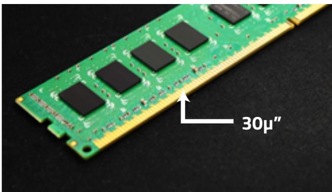
In order to ensure the quality of the signal transmission between the connector and ATP DRAM module, ATP utilizes gold finger plating with  $30\mu$  thickness, compared to competitors' DRAM modules thickness typically at less than  $10\mu$ .
